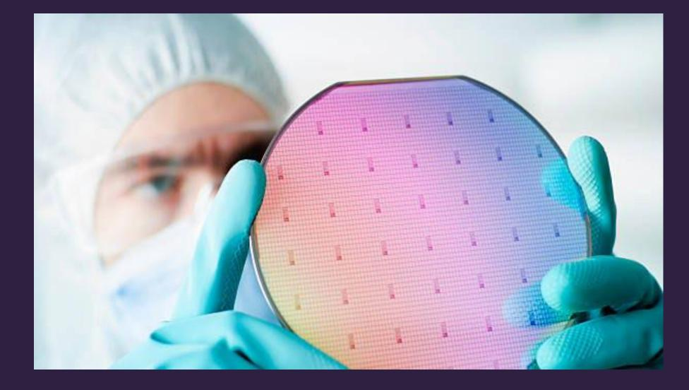
Current alcohol (Isopropanol) used for cleaning has impurities in it (primarily Sulfur). Sulfur is a known defect-causing contaminant on etched wafers.
